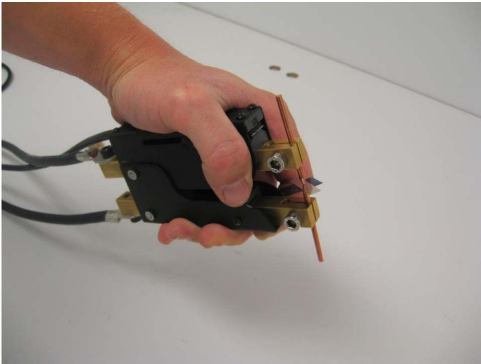
FIGURE 5: The Moderate Power (PA-THP) being used to weld a thin strip of sheet metal.
