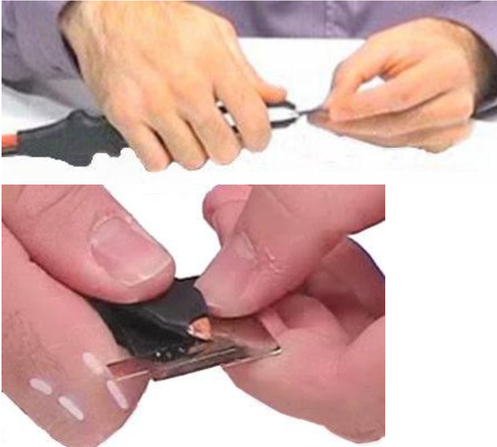
FIGURE 3: The tweezer hand piece (THP) being used to weld thin sheet metal.
